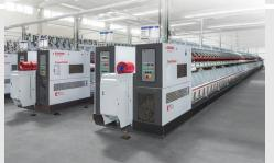
Twisting and direct cabling machines for all kind of carpet and hand knitting yarns
