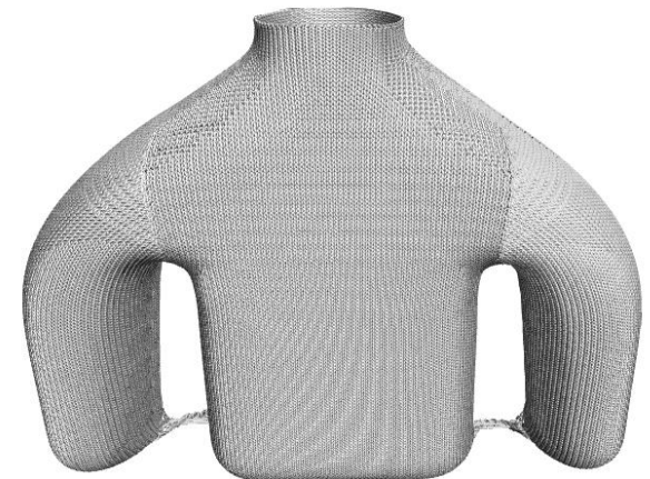
3D simulation of the stitch linking
