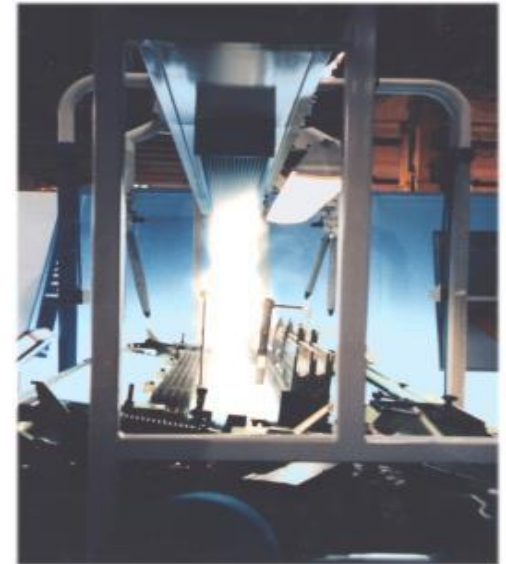
Laminar air flow of Loomsphere, demonstrated by smoke
